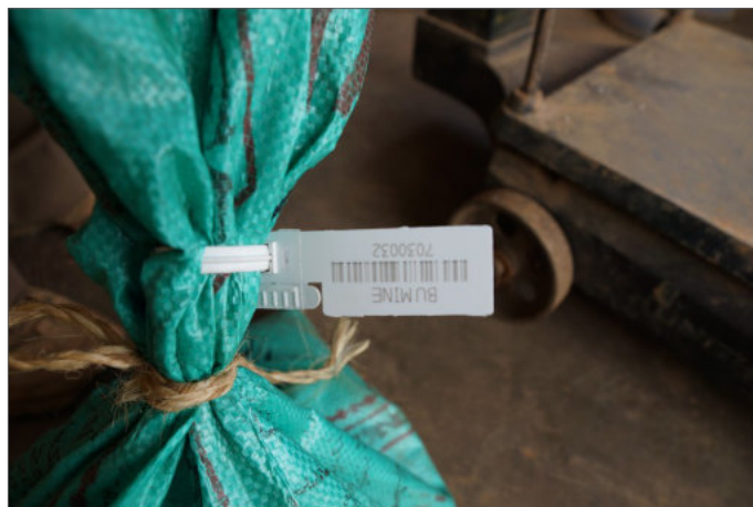
Once the dry concentrate is bagged and weighed, it is tagged and logged ready for sale to a local trader ( comptoir ) who will combine it into a larger blended lot for export to a processor/smelter.
