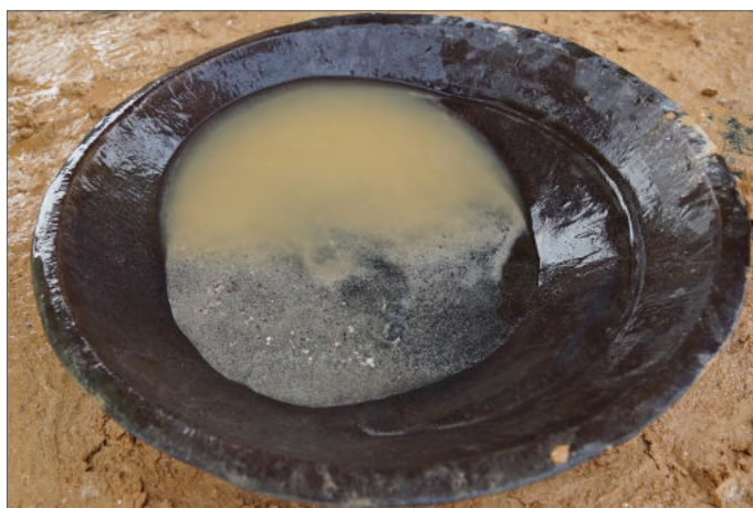
The material recovered from washing is a fine, dark-grey material that will contain 20-40% \text{Ta}_2\text{O}_5 .
