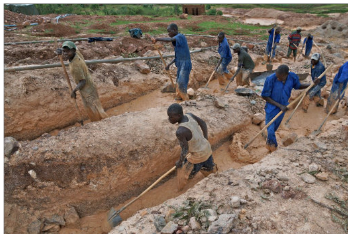
The first wash is often relatively crude. Plentiful and/or well-managed supplies of washing water is a critical factor for ASM operations.
