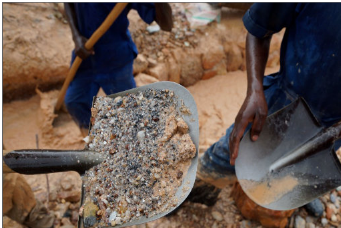
The mined ore is washed in stages to concentrate the relatively heavy fractions of tantalite.
