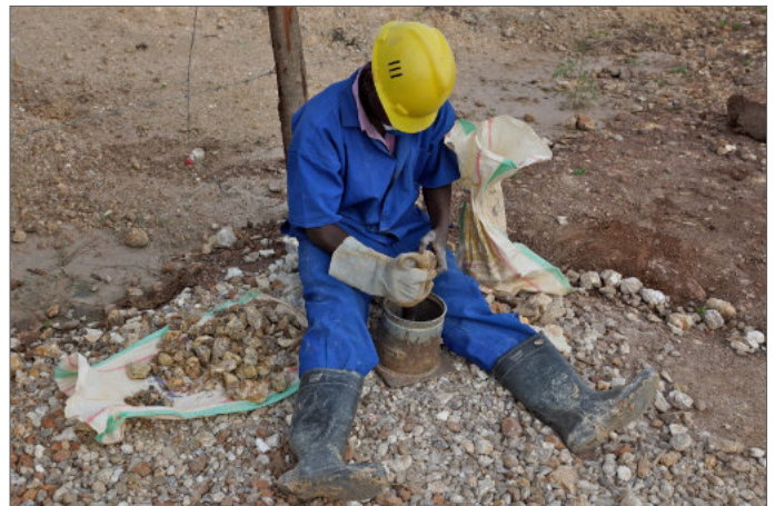
The extracted ore is typically a sandy gravel. Larger pieces are crushed manually or mechanically .
