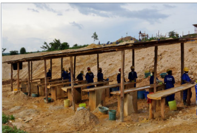
Subsequent stages might include manual washing tables (shown here) or mechanised gravity jigging tables.
