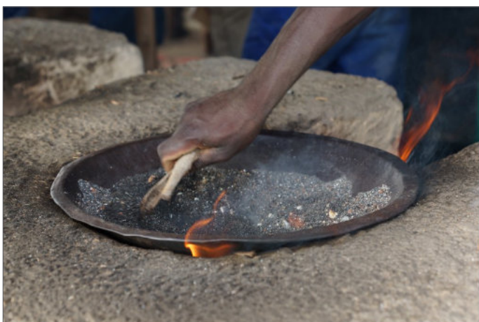
The concentrate is heated and dried to remove all moisture.
