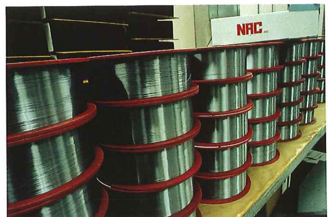
Tantalum wire produced at HCST Newton
