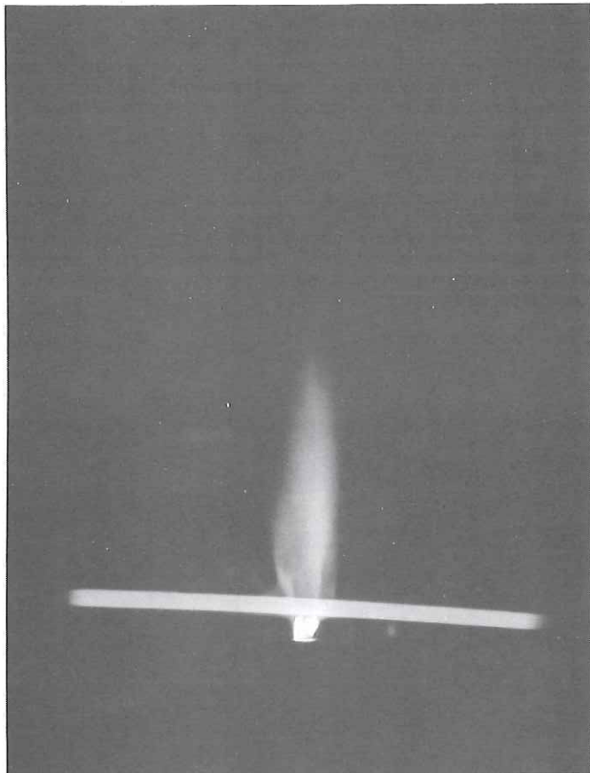
Figure 2: AC-103 alloy (Nb-10Hf-1Ti) heat pipe is heated directly in the 2800°C flame of an oxygen/mapp gas torch. To protect the surface of the C-103 from oxidation at high temperature, a protective silicide coating has been fused to the exterior surface. The pictured heat pipe measures approximately 30 cm long by 1 cm cross-section. The inside of this pipe is lined with porous niobium alloy approximately 0.6 mm thick. Lithium is the working fluid.
