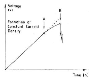
The exact determination of the scintillation point would be most interesting as far as the use of tantalum powder is concerned, since this determines the maximum formation voltage with which the sintered anode can be charged.
