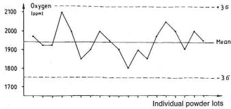
This type of presentation in the form of a control chart can be used for any other parameter, such as capacitance or grain size.
