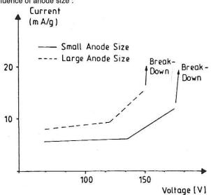
This testing method was applied in the previously mentioned examples to the formation of a sintered anode, but it can also be applied in a modified form to already formed anodes in order to test the quality of the oxide film.
