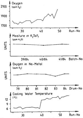
In this case only the temperature of the coolant changed synchronically with the oxygen content, and so the increase in oxygen was eliminated by adding an improved cooling system.
