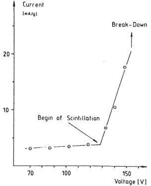
One can easily recognise the two points of the BDV-curve, the beginning of scintillation (A) and the break-down voltage (B).
