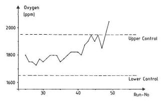
There were some production and raw material parameters which were most likely to be contributing to this oxygen content increase, namely the humidity in  $\rm K_2TaF_7$ , the oxygen content in the sodium and the temperature of the cooling water.
