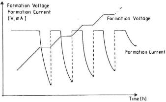
The formation currents of each step at the end of each holding period can be plotted against formation voltage:
