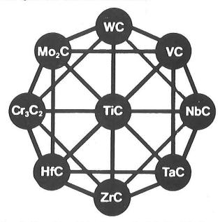
From all of the cubic carbides shown on the right side of the diagram, TiC acts as the host lattice for the mixed carbide phase and is, therefore, added more or less regularly together with TaC.
