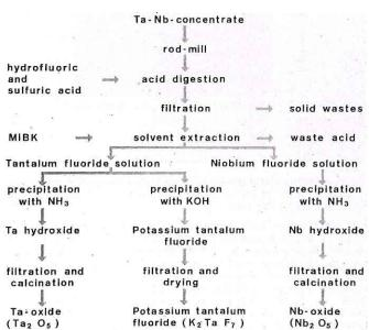
This product line, which produced the first  $K_2TaF_7$  commercially in 1952, has undergone several modification and expansion programs in the intervening years. The latest was during 1978 to 1982 to increase the capacity of the digesters and the  $Ta_2O_5/Nb_2O_5$  out-
