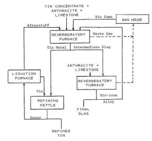
With 70 tons of high grade Malaysian tin concentrate in the charge, approximately 7 tons of final slag will be produced. Since essentially all the tantalum in the concentrate will be in the final slag, there is a concentration ratio of 10:1 for the tantalum during the tin smelting operation.
