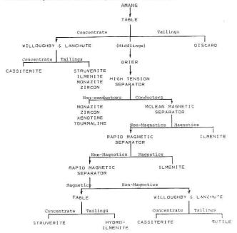
The separation of the minerals is based on their physical properties: struverite, for example, is magnetic, but less magnetic than ilmenite, it is a conductor of electricity and it is fairly heavy but less so than cassiterite. These properties are exploited to their full extent by the amang plant operators.
