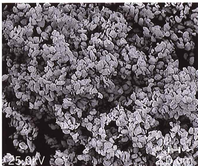
Figure 1: SEM image of HDH niobium powder
