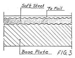
To clad with tantalum as light as 0.15 mm (0.006 in.), an interface of about 1 mm (0.040 in.) thickness would be used. When fusion welding is required to join composite plates, a copper interface is often used to disperse by conduction the heat of welding.
