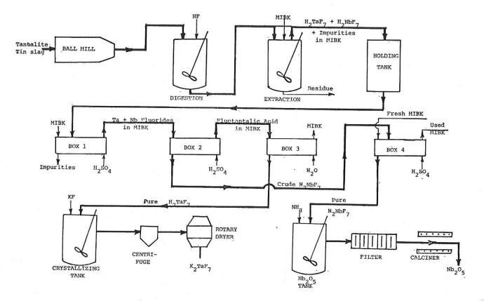
ther liquor is pumped off and the precipitate washed to remove fluorides. After filtering, the resulting cake is calcined at 875° to 975 °C, producing high purity niobium oxide.
