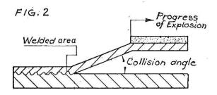
The reaction is so rapid that very little heat is generated and, although welding is effected, the materials never get hot enough to create significant difference in thermal expansion between the two metals. Thus the brittle intermetallic alloy formed in the weld zone does not fracture after cooling.
