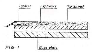
Upon detonation, the explosion occurs progressively across the sheet at a very high speed. The explosion force accelerates the tantalum sheet toward the base plate at a very high speed with tremendous force, causing it to progressively impact the base plate at a defined collision angle (Fig. 2).
